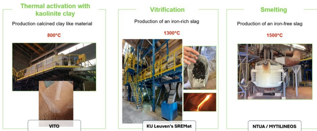
Figure 4. ReActiv processing routes to develop BR-based SCMs.
